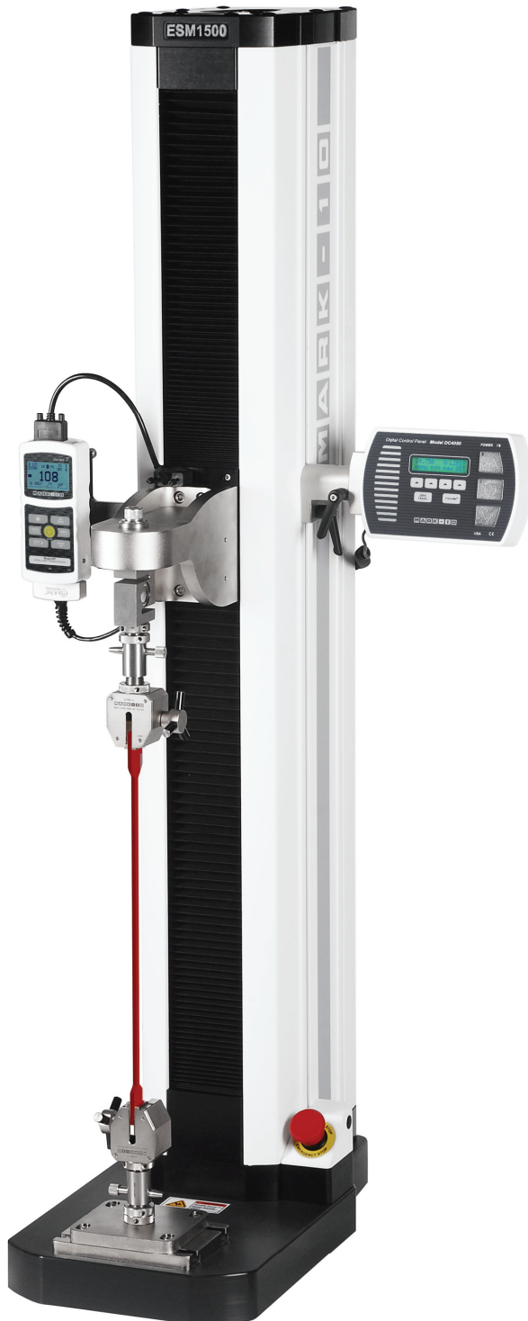
^ ESM1500LC is shown above configured for a tensile test, with a Series R01 force sensor, Model 7i indicator, G1061-2 wedge grips, and eye end adapters.
