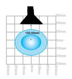
Diagrams above highlight the capture area of the stay put arms when extracting at a flow rate of 60m³/hr (darker shading) and 100m³/hr. These measurements were taken with the arm situated above the working area.
