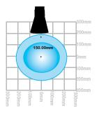
Diagrams above highlight the capture area of the stay put arms when extracting at a flow rate of 30m<sup>3</sup>/hr (darker shading) and 50m<sup>3</sup>/hr for 32mm arms and 120m<sup>3</sup>/hr (darker shading) and 190m<sup>3</sup>/hr for 75mm arms. These measurements were taken with the arm situated above the working area.
