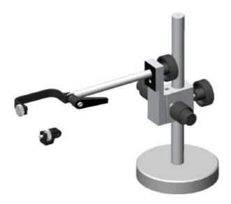
**OP-006 267 is a portable boom stand with precision extra fine rack & pinion Z-movement**, specially developed for using with Flexia family of video microscopes. Flexia can be tilted 90° up, 90° down and also 360° laterally on this stand. One extra 180° rotational adapter and one horizontal extension rod is included in delivery kit for more flexibility.
