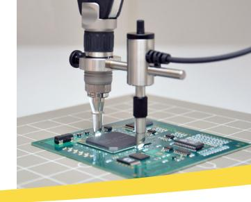
State of the art BGA Lenses with a range of Side-view Probes for reliable Visual Inspection of solder joints of BGA, uBGA, CSP and Flip-Chip packages with stand-off down to 0.04 mm (40 microns). The interchangeable Optical Probes are key elements in the Optilia BGA Inspection system and are easily attached to Flexia 5.0 mega pixel Digital Video Inspection Microscopes.
