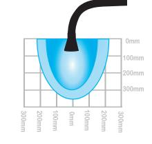
Capture area of 'Stay Put' arm when extracting at a flow rate of 60m<sup>3</sup>/hr (darker shading) and 100m<sup>3</sup>/hr with the arm resting on the work surface.
