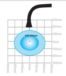
Capture area of 'Stay Put' arm when extracting at a flow rate of 60m<sup>3</sup>/hr (darker shading) and 100m<sup>3</sup>/hr with the arm situated above the working area.
