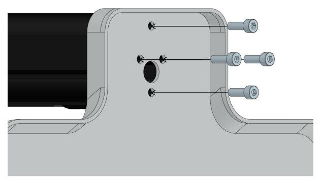
2. Install the Microscope Support Adapter on the Rack and Pinion Unit, and tighten the three screws.
