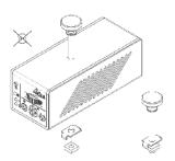
Up to 2 HiPower spots and 1 LED product with 40 LEDs (e.g. Ringlight 66/40 or backlight) can be connected to this control unit. It can be used as a table mounted device or with special microscopes by fastening it to the column by means of the screw included.
