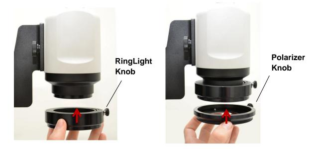
3. Direction of Polarization Filter 1 can be adjusted by turning the Rotational Ring, below picture.
