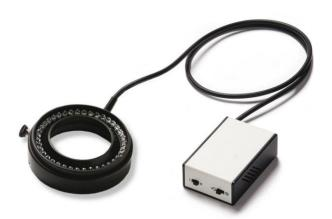
Ring-light containing 40 white LEDs for bright and homogenous illumination of objects. Designed for assembly on Optilia W10x-HD, W20x-HD and M20x-HD cameras. The compact control unit features an ON-OFF switch, brightness control and two outputs for connection to LED illumination units. With optional Segment control unit, user can toggle 4 groups of LEDs clockwise or anticlockwise.
