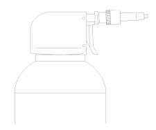
Screw the nozzle on to the adapter of the cleaning spray and spray. If the nozzle opening is clogged use the enclosed cleaning wire and push it through from the inside out.
