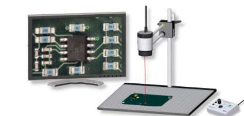
Configuration A: Stand-alone HD Camera with Control Unit and 22" Full HD monitor.
