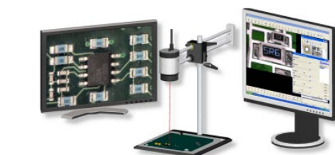
Configuration B: HD Camera with 22" Full HD monitor connected to PC and Optilia Picsara software.
