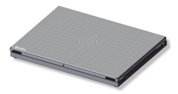
**OP-006 500** is a linear floating XY-translation stage, equipped with thick static dissipative top matting. Ball bearing slider design of the unit permits low friction linear movement with no backlash or side-play. This precision stage provides controlled point-to-point lateral movement along two linear axes. A detachable \$4mm mating plug with 1m flying end wire is included for earth connection.
