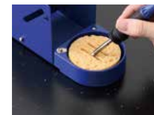
Manual cleaning with wet sponge
