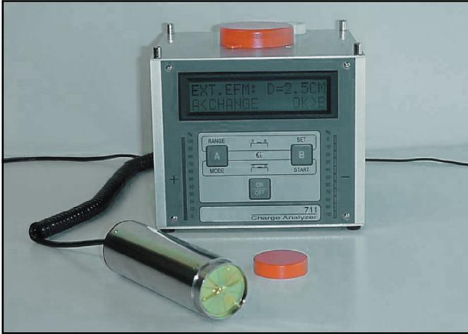
Figure 11. Remote Field Sensor Probe Operation.
