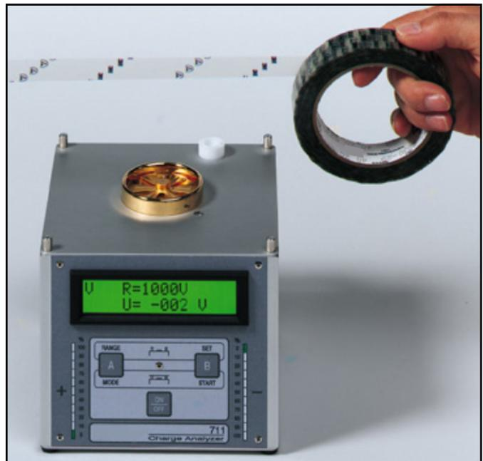
Figure 3. Testing Low Tribocharging Tapes.
