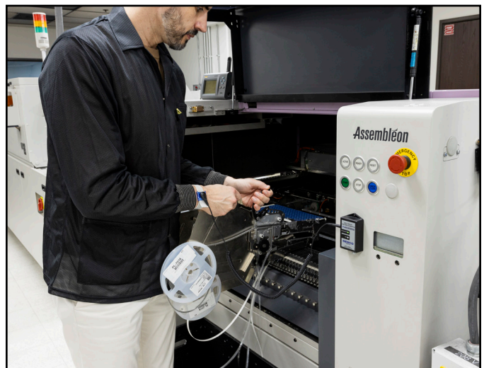
Figure 8. Using the Multi-Mount Continuous Monitor at a machine workstation
