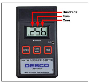
Figure 5. Reading the Digital Static Field Meter while in the ±2kV range
