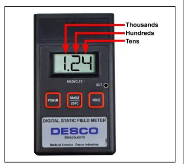
Figure 4. Reading the Digital Static Field Meter while in the ±20kV range
