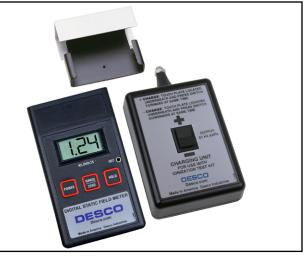
Figure 1. Desco 19493 Ionisation Test Kit
