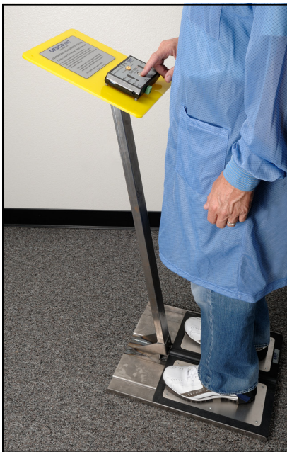
Figure 12. Using the EMIT 50415 Stand with the Dual Independent Tester
