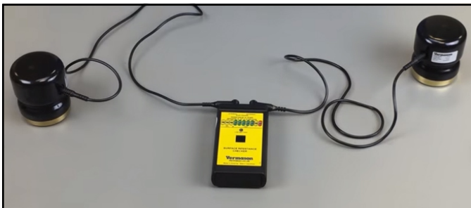
Figure 5. Using the test leads and 2.27 kg electrodes to measure Rp-p
