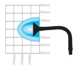
Diagrams above highlight the capture area of the stay put arms when extracting at a flow rate of 60m³/hr (darker shading) and 100m³/hr. These measurements were taken with the arm resting on the work surface.
