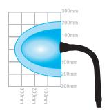
Diagrams above highlight the capture area of the stay put arms when extracting at a flow rate of 30m³/hr (darker shading) and 50m³/hr for 32mm arms and 120m³/hr (darker shading) and 190m³/hr for 75mm arms. These measurements were taken with the arm resting sideways on the work surface.
